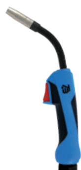
TBi 150 Expert Classic Series 60% (10 min.) Mix: 150 A CO 2 : 170 A Ø 0.6-1.0 mm
