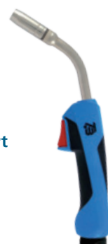
TBi 250 Expert Classic Series 60% (10 min.) Mix: 200 A CO 2 : 230 A Ø 0.8-1.2 mm
