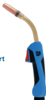
TBi 240 Expert Classic Serie 60% (10 min.) Mix: 210 A CO 2 : 220 A Ø 0.8-1.2 mm
