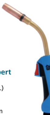
TBi 360 Expert Classic Series 60% (10 min.) Mix: 300 A CO 2 : 330 A Ø 1.0-1.6 mm
