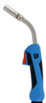
TBi 241 Expert Classic Series 100% (10 min.) Mix: 270 A CO 2 : 300 A Ø 0.8-1.2 mm
