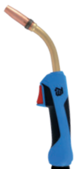
TBi 241 Expert Classic Series 100% (10 min.) Mix: 270 A CO 2 : 300 A Ø 0.8-1.2 mm
